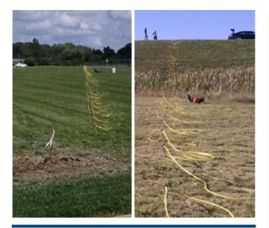
CTL ENGINEERING HAS THE ABILITY TO PROVIDE GEOPHYSICAL TESTING INCLUDING 2D & 3D ELECTRICAL RESISTIVITY AND INDUCED POLARIZATION SURVEYS TO ASSIST IN PERFORMING NON-DESTRUCTIVE SUBSURFACE EXPLORATIONS.
