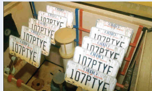
Salt Spray Testing for Corrosion Resistance
